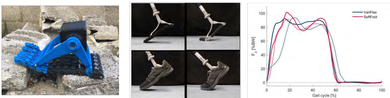
Figure 1 On the left, SoftFoot prototype for robots. In the middle, a comparison between a prosthesis with a rigid sole and the SoftFoot prosthesis [5] . The SoftFoot also offers a more natural aesthetic, even with shoes. On the right, sagittal force measured by a load cell placed between the prosthetic foot and the walking boot worn by a healthy subject. The force profile when stepping on an obstacle (dotted line) with the SoftFoot (red line) remains closer to that for level walking (solid line) than with the VariFlex (an Össur carbon foot - blue lines), and it is on average greater than that of the VariFlex.
